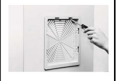
Place filter mat inside filter housing then insert filter louvre into filter body and insure that they snap tightly together.
